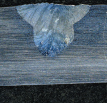
Fusion depth measurement of welding and riveting
